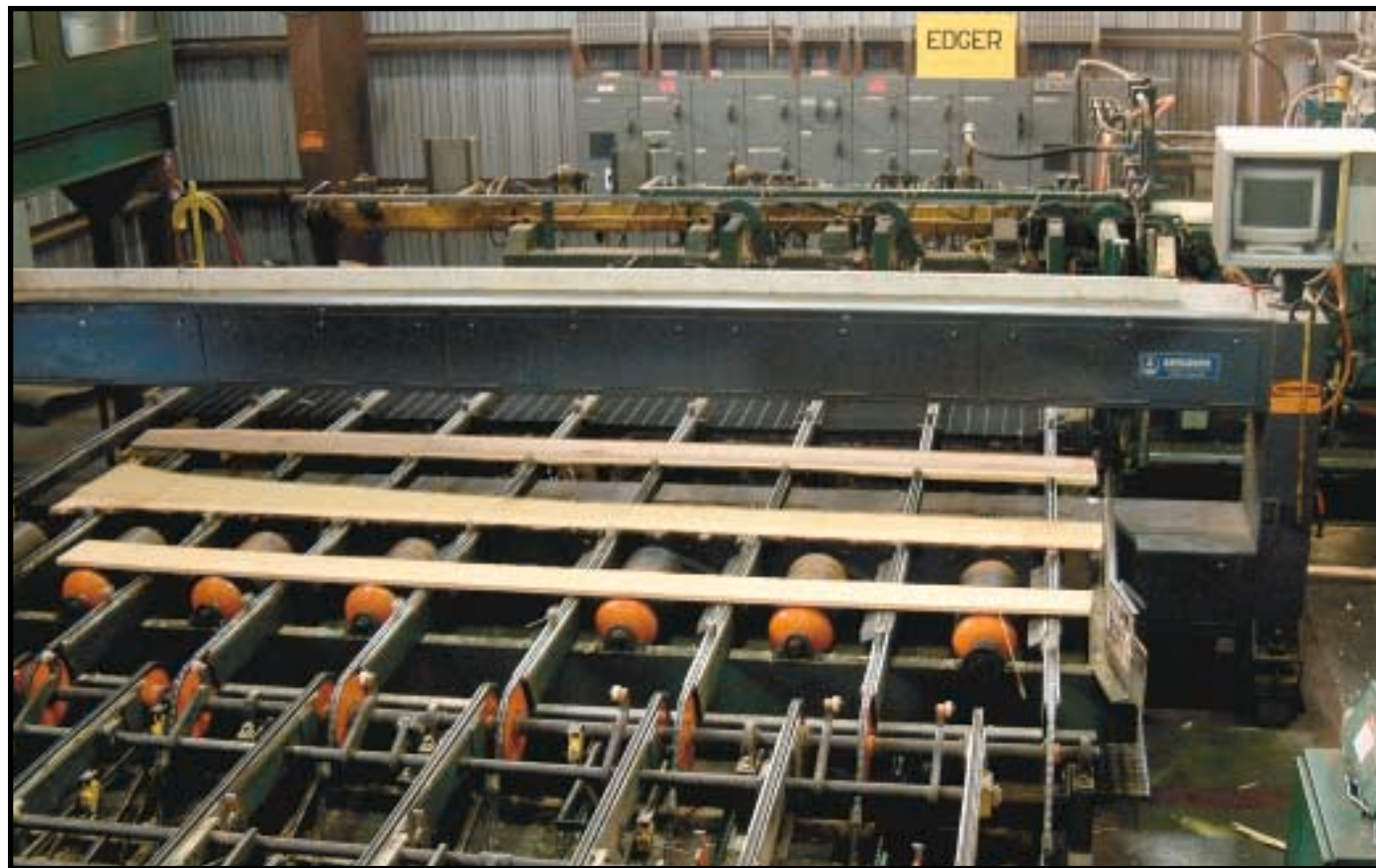
USNR edger optimizer reads lumber for three-saw edger.
